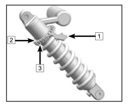
Rear shock absorber: K2C Rear shock absorber volume: 220 ± 2 mL
