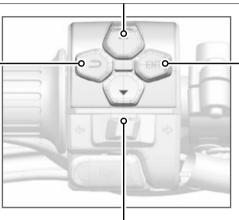
For Main interface: press it to enter the first-level menu, and long press it to play the song (when Bluetooth is connected).
