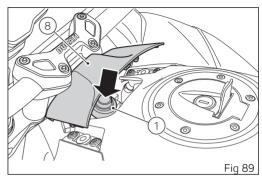
(Fig 89) indicates the position of the Hands Free unit (1), with protection lid (8) and (Fig 90) indicates the position of the antenna (2) under panel (9) at the key symbol.
