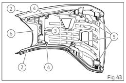
Position the passenger seat on the motorcycle. Now the seat is in a lowered position.
