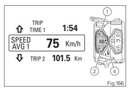
If you press button (1) or (2), the instrument panel will display SPEED AVG 1 again, without resetting the value.
