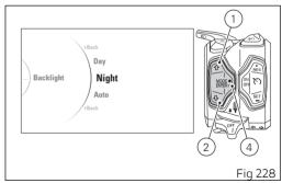
Select NIGHT (night more) to permanently set display black background for dimmed visibility - recommended in case of poor ambient light and/or at night.
