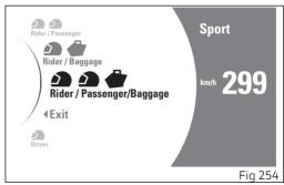
Every load setup is associated with a specific front fork rebound and compression damping, a specific rear shock absorber rebound and compression damping as well as a specific rear shock absorber spring preload that changes according to the Riding Mode.
