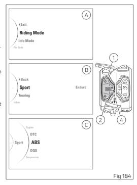
When you access the function, all possible customisation levels (levels from 1 to 3 and OFF status) are listed on the left and the set ABS level or status is shown on the right.
