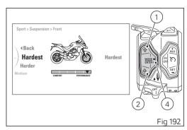
corresponding paired value in the central table (highlighted with a black arrow ▼) will be displayed. Once the desired level is highlighted, press button (4) to memorise the new selection.
