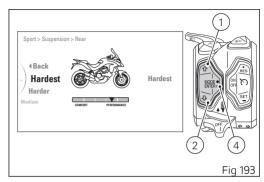
With button (1) or (2) select the new level of intervention desired. For each highlighted level, the corresponding paired value in the central table (highlighted with a black arrow ▼) will be displayed. Once the desired level is highlighted, press button (4) to memorise the new selection.
