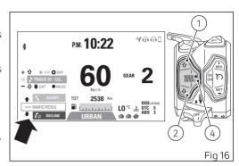
To activate the Recall function within the 5 seconds, press button (1).
