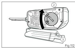
Insert the new battery (3) into the battery compartment with the slot (2) facing upwards. Using a coin of appropriate size applied to the slot (2), rotate the battery (3) anticlockwise to fix it (as indicated by the "CLOSE" indication on the battery).
