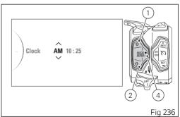
once you reach the desired value, press button (4) to confirm: the arrows move to the "minutes" value to allow setting it.
