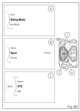
When you access the function, all possible customisation levels (levels from 1 to 8 and OFF status) are listed on the left and the set DTC level or status is shown on the right.
