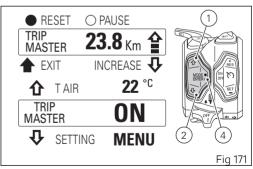
To disable the Trip Master function, scroll down the Menu by pressing buttons (1) and (2) up to "TRIP MASTER ON" and press button (4). In this way, the instrument panel interrupts the function and resets the count.
