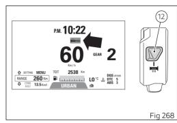
Level selection with Heated Handgrips "off": Even if heated handgrips are turned off, it is still possible to set them to LOW, MED or HIGH level, but the icon will have a white background in DAY backlighting option of the instrument panel, or black in NIGHT backlighting option of the instrument panel.
