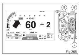
When the new requested target speed is not modified for over 5 seconds, the SET icon is displayed again.
