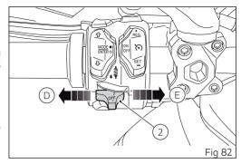
Automatic switch-off feature can be disabled through the specific option within the SETTING MENU. For further details, refer to paragraph Turn indicator automatic switch-off feature (TURN INDICATORS OFF) page 292.
