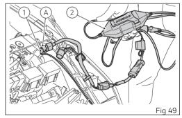
maintenance kit) since its electronics monitors the battery voltage and features a maximum charge current of 1.5 Ah. Connect the battery maintainer to the diagnostic socket.
