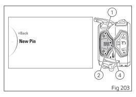
After accessing the Pin Code entering function (New Pin), the instrument panel displays "New Pin" with spaces allowing to enter the four digits of the new Pin code to be entered: "0" and "---". The two arrows on the digit give the possibility to set it.
