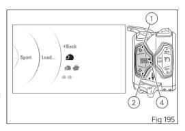
If you select a setup to be customised, when you access the function, all possible customisation levels (levels from 1 to 24) are listed on the left and the currently set level is shown on the right.
