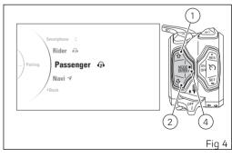
The instrument panel displays "Wait..." during device search phase. The pairing ends automatically when devices are detected within the range. This search phase takes 60 seconds.
