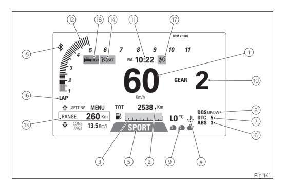
Data displayed on the main screen for FULL layout 21) Fog lights (if any). are as follows:
