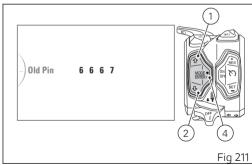
When you press button (4) to confirm the fourth and last digit, the instrument panel responds as follows:
