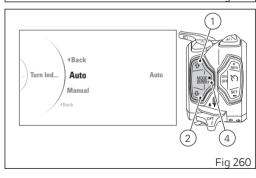
Once the desired function is highlighted, press button (4) to set the selected mode.
