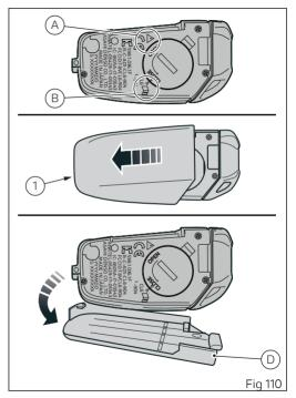
Remove the rear plastic shell (1) of the grip by pushing it forward and lifting it as shown in the figure.
