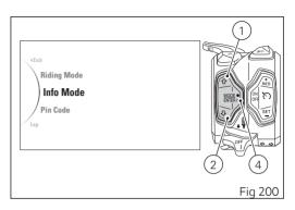
After entering the function, the display shows the available Info Modes ("Track", "Full", "City" and "Off Road") on the left side and set Info Mode on the right side. Within this page, the instrument panel displays the following indications:
