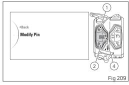
After accessing the Pin Code change function (Modify Pin), the instrument panel displays "Old Pin" with spaces allowing to enter the four digits of the set Pin code. "O" and "- - - -". The two arrows on the digit give the possibility to set it.
