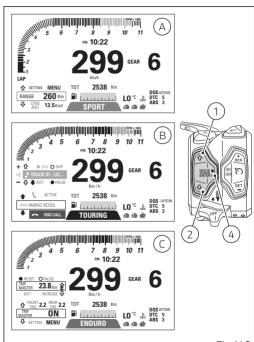
During the first 1000 km (600 mi) of the odometer (vehicle break-in period) a "virtual" engine rpm limiter is displayed. The "orange area" of rev counter starts from 6000 rpm. We recommend the user not to reach this orange area during break-in period. After the break-in period, the "virtual" limiter indicates and advises the rider to ride at lower revs when the engine is cold. The "virtual" limiter changes according to the engine temperature.
