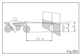
Procedure for adjusting low beam/high beam along the vertical axis
