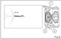
The instrument panel shows "Pairing": to confirm the selected device Pairing press button (4) again. If you do not wish to proceed with pairing, highlight the " ■ Back" indication and press button (4). By confirming the device pairing, the instrument panel will display "Wait...".
