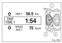
While if you press button (4), value for TRIP TIME 1 will be reset and the instrument panel will display TRIP TIME 1 at "0:00".
