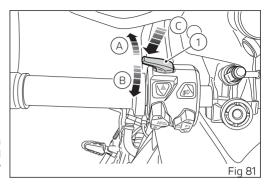
Function for switching the Cornering lights on/
