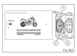
With buttons (1) and (2) select the new level of intervention desired. For each highlighted level, the corresponding paired value in the central table (highlighted with a black background or arrow ▼) will be displayed.
