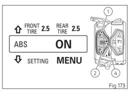
If the ABS is disabled, the instrument panel shows "ABS OFF" and ABS light on. Once "ABS OFF" is displayed, press button (4) to enable the ABS.
