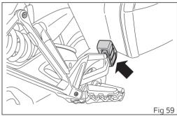
Push forward (towards the front wheel) until fully home; only in this position will it be possible to lower handle (A) and lock pannier in place, this operation ensures pannier locking to its mounting points. Turn the key counter clockwise to lock handle and remove it.
