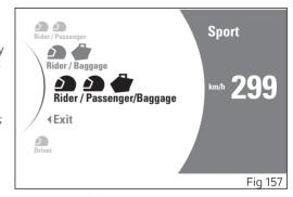
Press button (2) for one second to activate the load mode function menu.
