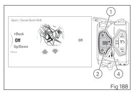
With buttons (1) and (2) select the new level of intervention desired. For each highlighted level, the system intervention level (highlighted with one and/ or two black arrows) will be displayed.
