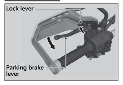
Place your vehicle on a firm, level surface. Stop the engine and push your vehicle while the parking brake is set to check the efficacy of the parking brake.
