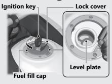
Do not fill with fuel above the level plate. Fuel type: Unleaded petrol only Fuel octane number: Your vehicle is designed to use Research Octane Number (RON) 91 or higher.
