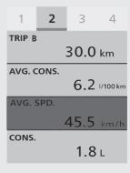
To reset the tripmeter B average speed [AVG. SPD.]: P.72
