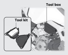
Removing the tool box P.277
