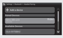
Select [Designate as a Rider] or [Connect Headset], and then press the ENT switch to [ON] (enable) the function.
