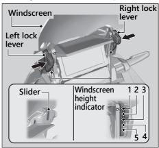
If the windscreen does not move smoothly, clean the sliders using a sponge or a soft towel with neutral detergent to remove dust.
