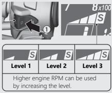
The selected level is maintained even when the ignition switch is turned to the OFF position, or transmission is switched to out of S mode.
