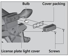
Install a new bulb and parts in the reverse order of removal.
