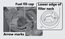
Do not fill with fuel above the lower edge of the filler neck
