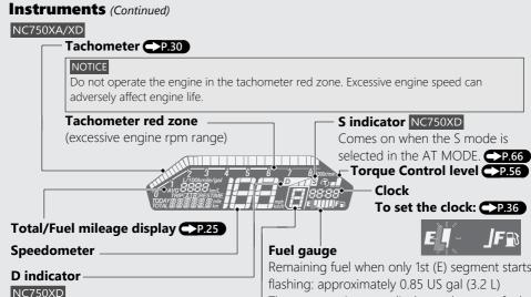
Remaining fuel when only 1st (E) segment starts flashing: approximately 0.85 US gal (3.2 L) The reserve tripmeter display and reserve fuel consumption display show at the same time.
