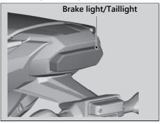
The brake light and taillight uses several LEDs. If there is an LED which is not turned on, see your dealer for servicing.
