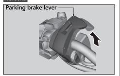
Place your vehicle on a firm, level surface. Stop the engine and push your vehicle while set the parking brake to check the efficacy of the parking brake.
