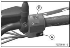
A. Starter Button **B. Engine Stop Switch**
