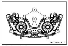
A. Horizontal Adjusters **B. Vertical Adjusters**
