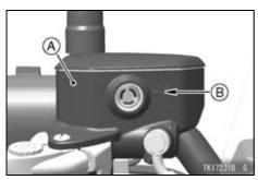
A. Front Brake Fluid Reservoir B. Lower Level Line
