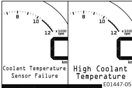
**Coolant Temperature Sensor Failure** appears on the display if the coolant temperature sensor is faulty.
