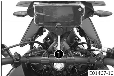
Socket **1** for electrical accessories is fitted in front of the upper triple clamp. It is connected to the ignition plus and is fuse-protected.
