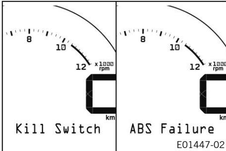
**Kill Switch** appears on the display if the emergency off switch is pressed.
