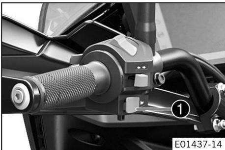
Horn button ❶ is fitted on the left side of the handlebar.
