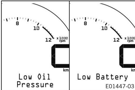
**Low Oil Pressure** appears on the display if the oil pressure is too low.
