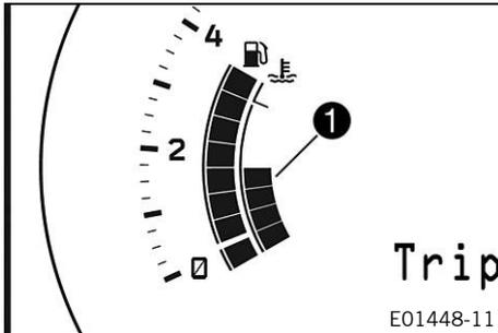
The coolant temperature is shown in area **1** of the display. The coolant temperature indicator consists of bars. The more bars that light up, the hotter the coolant.
