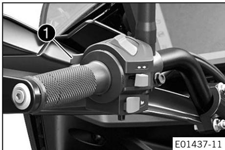
High beam flasher button ❶ is fitted on the left side of the handlebar.
