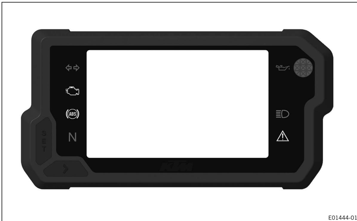
The indicator lamps offer additional information about the operating state of the motorcycle. When the ignition is switched on, all indicator lamps light up briefly except for the turn signal indicator lamp. As soon as a warning for operating safety has been detected, the general warning lamp
