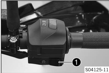
Start button ① is fitted on the right side of the handlebar.
