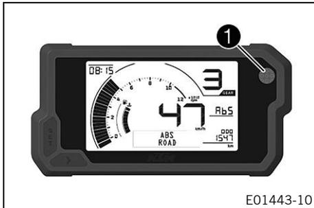
The shift warning light **1** is at the top right of the combination instrument.
