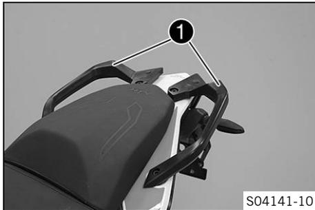
The grab handles ❶ are used for moving the motorcycle around. If you carry a passenger, the passenger can hold onto the grab handles during the trip.
