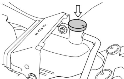
2. Remove the filler cap and add specified engine coolant through the filler hole until it reaches the "F" line. Refer to the FUEL, ENGINE OIL AND COOLANT RECOMMENDATIONS section.
