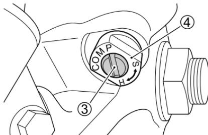
To set the compression damping force adjuster to the standard position, turn the adjuster clockwise until it stops and then turn it counterclockwise 8 clicks.
