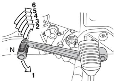
This motorcycle has a 6-speed transmission which operates as shown. To shift properly, squeeze the clutch lever and close the throttle at the same time you operate the gearshift lever. Lift the gearshift lever to upshift and depress the lever to downshift. Neutral is located between 1st and 2nd gear. When neutral is desired, depress or lift the lever halfway between 1st and 2nd gear.
