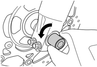
9. Turn the axle shaft counter-clockwise and draw it out.
