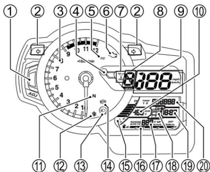
The malfunction indicator light ⑥, freeze indicator light ⑫, engine coolant temperature indicator light/oil pressure indicator light ④, ABS indicator light ⑭, traction control indicator light ⑤, LCD's and tachometer needle work as follows to confirm their function when the ignition switch is turned to the "ON" position.
