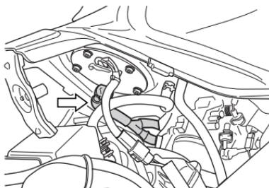
Inspect the fuel hose for damage and fuel leakage. If any defects are found, the fuel hose must be replaced.
