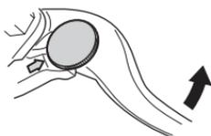
The distance between the throttle grip and the brake lever is adjustable to 5 positions.
