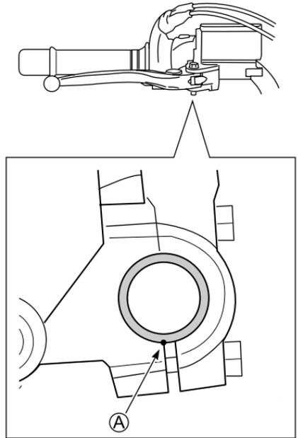
Align the dot mark on the handlebar with the mating surface of the lever holder (A).
