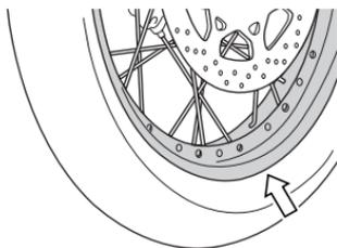
Check to see if there is any damage like crack, distortion or bend in the wheel rim.
