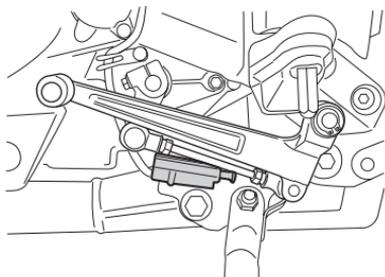
Check the side stand/ignition interlock system for proper operation as follows:
