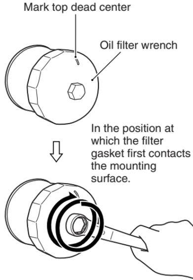
Tighten the filter 2 turns or to specified torque.
