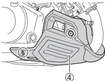
4. Remove the right and left bolts and remove the under cowlings ④.
