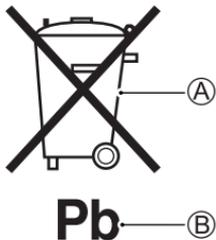
The crossed-out wheeled bin symbol (A) located on the battery label indicates that an used battery should be collected separately from ordinary household waste.
