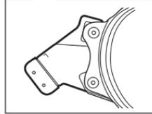
8. Slide the right and left fuel tank side covers ④ forward to slip off the hook. Remove the right and left fuel tank side covers ④.
