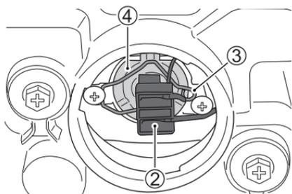
2. Disconnect the socket ②. Unhook the bulb holder spring ③ and pull out the bulb ④.
