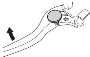
The distance between the grip and the clutch lever is adjustable to 4 positions. To change the position, push the clutch lever forward and turn the adjuster to the desired position. When changing the clutch lever position, always be sure the adjuster stops in the proper position; a projection of the clutch lever pivot should fit into the depression of the adjuster. This motorcycle is delivered from the factory with its adjuster set on position 2.
