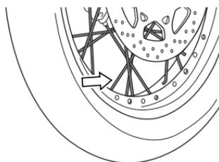
Check the tension of spokes to verify the tightness of the spoke nipples. The tension can be checked by hitting the spokes with a small metal bar. If the spoke nipple is loose, its sound will be dull.
