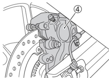
8. Remove the rear brake caliper assembly (4).
