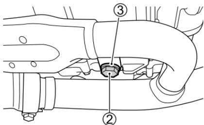
3. Remove the drain plug ② and gasket ③ from the bottom of the engine and drain the engine oil into a drain pan.
