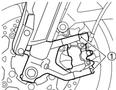
3. Remove both brake calipers from the front forks by removing two mounting bolts ① on each of the calipers.
