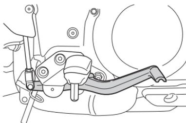
Depressing the rear brake pedal will apply the rear disk brake. The brake light will be lit when the rear brake is operated.
