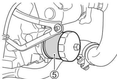
5. Turn the oil filter ⑤ counter-clockwise with a Suzuki “cap type” oil filter wrench or a “strap type” filter wrench of the proper size.
