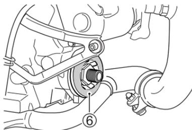
6. Wipe off the mounting surface ⑥ on the engine where the new filter will be seated with a clean rag.
