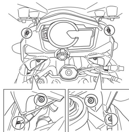
1. Remove the bolts and fasteners.
