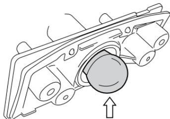
3. Push in on the bulb, twisting it to the left, and pull it out.
