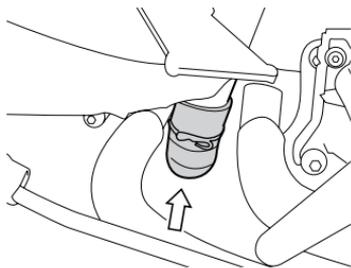
Remove the plug and drain water and oil at the periodic maintenance interval. The air cleaner drain plug is located beneath the air cleaner box.
