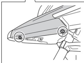
3. Remove the right and left bolts. Unhook the hooks and remove the right and left side covers ①.
