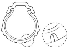
Check the condition of your tires each day before you ride. Replace tires if tires show visual evidence of damage, such as cracks or cuts, or if tread depth is less than 1.6 mm (0.06 in) front, 2.0 mm (0.08 in) rear.
