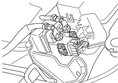
The main fuse is located under the seat. One 30A spare fuse is located in the starter relay box.
