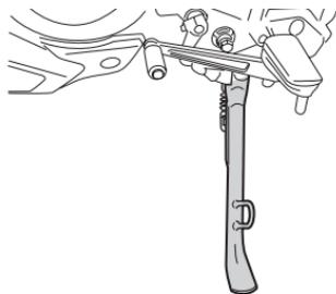
An interlock system is provided to cut off the ignition circuit when the side stand is down and the transmission is in any gear other than neutral.
