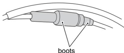
The throttle cable has boots. Check that the boots are fit securely. Do not apply water directly to the boots when washing. Wipe off dirt from the boots with a wet cloth when the boots are dirty.
