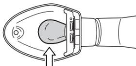
2. Push in on the bulb, twisting it to the left, and pull it out.
