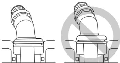
**NOTE:** Push the spark plug caps all the way on so that there is a tight seal.
