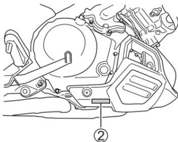
The frame number ① is stamped on the steering head as shown in the illustration. The engine serial number ② is stamped on the crankcase assembly.
