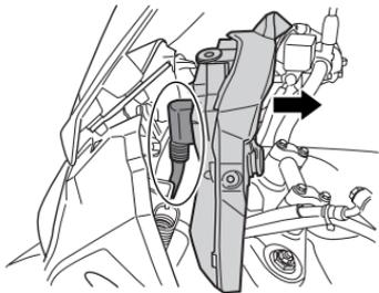
3. Move the instrument panel to the arrowed direction.
