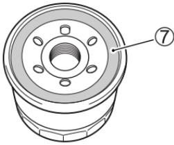
7. Smear a little engine oil around the rubber gasket ⑦ of the new oil filter.
