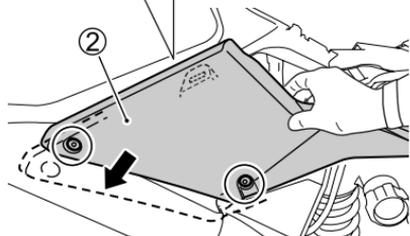
4. Remove the bolts. Pull the right and left side frame covers ②.
