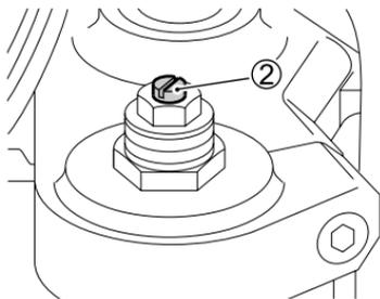
To set the rebound damping force adjuster to the standard position, turn the adjuster clockwise until it stops and then turn it counterclockwise 8 clicks.
