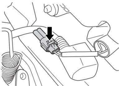
5. Disconnect the power source coupler. Remove the instrument panel assembly.
