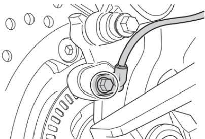
2. Remove the rear wheel speed sensor by removing the mounting bolt.
