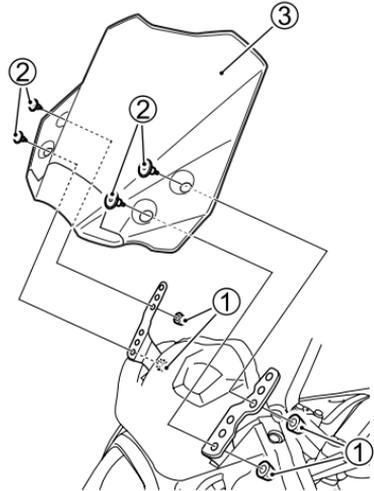
1. Remove the caps ① and bolts ② and then remove the windshield ③.
