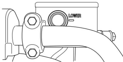
The clutch release mechanism of this motorcycle is operated by hydraulic pressure. There is no adjustment needed on the clutch release system because the system is self adjusting. However, inspect the following each time before driving to make sure that the system is in good condition and functioning properly.
