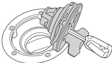
To open the fuel tank cap, insert the ignition key into the lock and turn it clockwise. With the key inserted, lift up with the key and open the fuel tank cap. To close the fuel tank cap, push the cap down firmly with the key in the cap lock.
