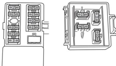
The fuses are located under the seat. Four spare fuses (one 10A, one 15A, one 3A and one 25A) are provided inside the fuse box cap.
