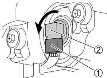
1. Disconnect the coupler ①. Turn the socket ② counter-clockwise and remove it.
