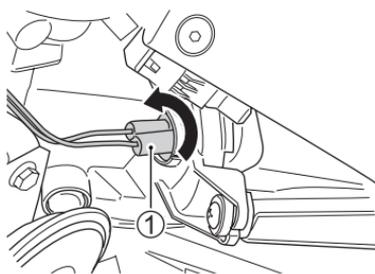
1. Turn the socket ① counterclockwise and remove it.
