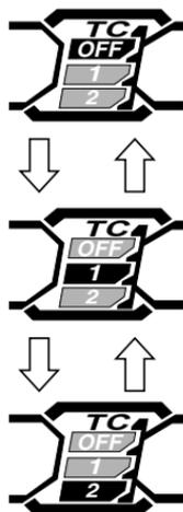
3. Press the traction control system switch ⑥ to cancel the mode selection. The traction control system display in the meter cluster returns to the normal display mode.
