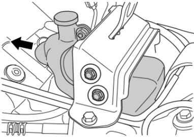
2. Remove the reservoir tank mounting bolts and move the reservoir tank forward.
