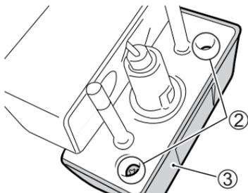
2. Remove the screws ② and take off the cover with the lens ③.
