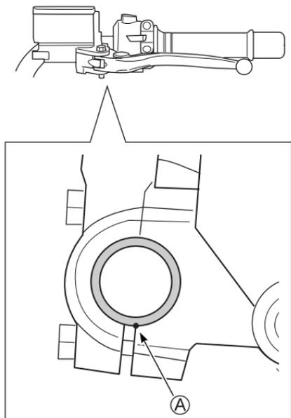
Align the dot mark on the handlebar with the mating surface of the lever holder **A**.
