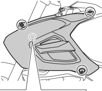
7. Remove the right and left fuel tank side covers bolts. Remove the wiring harness clamp.
