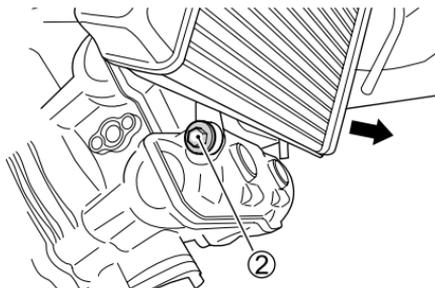
2. Remove the radiator mounting bolt ② and slide the radiator forward.
