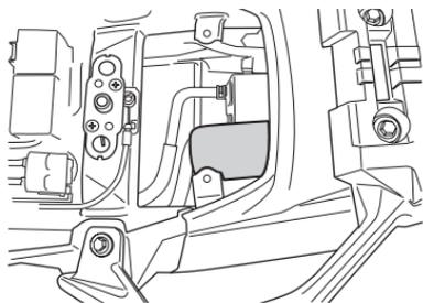
A tool kit is supplied and located under the seat.
