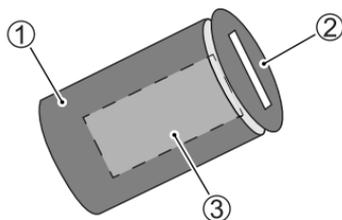
A lid ② is provided for the key cylinder ① to prevent tampering. Turning the lid position covers the keyhole ③, to prevent any alien substance entering the keyhole. To turn the lid, insert the tip of the key slightly into the lid and turn it.
