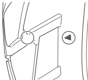
*NOTE: The “ $\Delta$ ” mark indicates the place where the wear bars are molded into the tire. When the wear bars contact the road, it indicates that the tire wear limit has been reached.*
