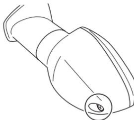
1. Remove the screw and take off the lens.
