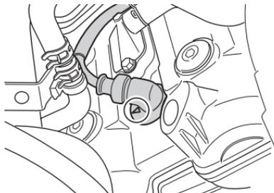
**NOTE:** When installing the spark plug caps, point the arrow marks on the spark plug caps to the exhaust side.
