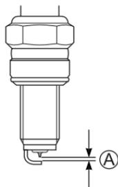
Measure the spark plug gap **(A)** with a wire type feeler gauge. The standard spark plug gap is 0.8 – 0.9 mm (0.031 – 0.035 in). If the measured spark plug gap is out of standard range, replace the spark plug with a new one.
