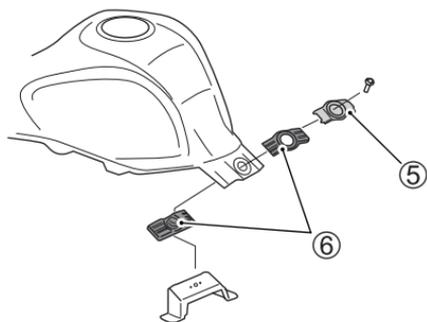
9. Remove the bolt. Remove the prop ⑤ and two cushions ⑥.
