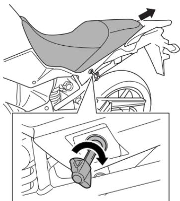
To remove the seat, insert the ignition key into the lock and turn it clockwise. Raise the rear end of the seat and slide it backward.
