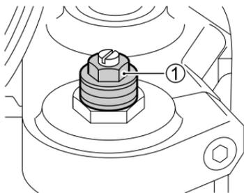
To change the spring pre-load, turn the adjuster ① clockwise or counterclockwise. Turning the adjuster clockwise will increase the spring pre-load. Turning the adjuster counterclockwise will decrease the spring pre-load.
