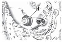
6. Loosen the axle stopper bolts 6.
