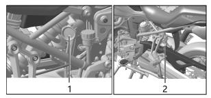
Driver only with 3 cases: Turn the adjustor 1 anticlockwise to limit, then turn it clockwise by 16±1 positions;
