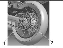
Locking torque of the rear axle nut:100±7N·m
