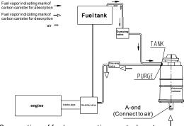
Connection of fuel evaporation control system
