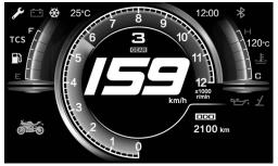
Driving gear position: The current gear position of engine. (Not neutral gear position).
