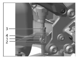
Free play for rear brake pedal shall be 15-25mm Fastening torque for nut of adjusting stud shall be 18 N.m
