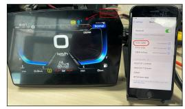
4.2 Open VOGE Global APP, Click icon of Bluetooth of (BLE-VOGE-) as beginning for connection, when successfully connected, the icon of Bluetooth will turn yellow, the instrument will show you the icon of Bluetooth 2, at this moment, click down-key on motorcycle's switch to shift to page on instrument of navigation.
