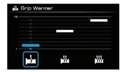
The three grip warmer presets can be customized here. Select a preset by operating the joystick left-right and adjust its heat level from 1-10 by operat-
