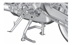
The operation of the centerstand and sidestand should be checked before each ride, and the pivots and metal-to-metal contact surfaces should be lubricated if necessary.
