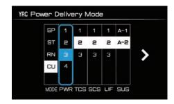
Select level 1 for sporty throttle response, level 2 for moderate throttle response, level 3 for mild throttle response and use level 4 for rainy days or whenever less engine power is desirable. (See page 3-15.)
