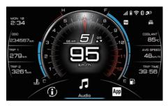
Smart features are accessed via the pop-up menu system at the bottom of the main display (see page 5-17). The menu system and all related features are controlled using the joystick/home button "๑๑" (see page 5-4).
