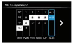
"SUS" can be set to A-1 and A-2. A-1 is a sporty setting with increased damping force, suitable for smoother road conditions. A-2 is a comfort setting with softer damping force, suitable for rougher road conditions. (See page 3-17.)
