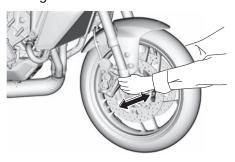
Checking the wheel bearings
