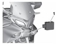
Millimeter-wave radar unit
