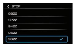
Select the r/min at which the shift indicator light will go off. The operational range is 6200–12000 r/min. It can be adjusted by 200 r/min increments. Confirm the settings by short pressing enter "✓" and return to the previous menu.
