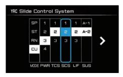
"SCS" can be set to 1, 2, and 3. Setting level 1 provides the least amount of system intervention, and setting level 3 provides the greatest amount of system intervention. (See page 3-16.)
