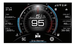
With this item highlighted, operate the joystick up-down to cycle between grip warmer OFF and 3 presets which can be customized in " Machine Settings"  $\rightarrow$  "Grip Warmer". (See page 5-29.)
