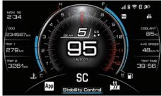
This option turns the stability control systems ("TCS", "SCS" and "LIF") on/off together. The stability control system indicator light "SC" will come on to indicate "SC OFF" status. (See page 5-8.)
