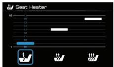
The three seat heater presets can be customized here. Select a preset by operating the joystick left-right and adjust its heat level from 1-10 by operating the joystick up-down. Confirm the settings by short pressing enter "✓" return to the previous menu.
