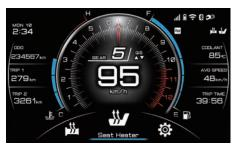
With this item highlighted, operate the joystick up-down to cycle between seat heater OFF and 3 presets which can be customized in "Machine Settings"  $\rightarrow$  "Seat Heater". (See page 5-29.)
