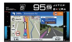
This vehicle is equipped with a navigation system which provides visual and audio (Bluetooth headset required) route guidance. To use the navigation system, you must first download the Garmin Motorize app from an application store onto your smartphone and then register for its paid service.
