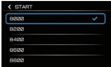
Select the r/min at which the shift indicator light will come on. The operational range is 6000–11800 r/min. It can be adjusted by 200 r/min increments. Confirm the settings by short pressing enter "
