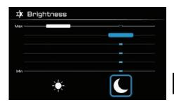
The multi-function meter is equipped with a sensor to detect ambient lighting conditions and adjust the display between day/night presets. The preset brightness levels can be customized here.
