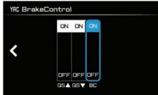
OFF: Only the standard anti-lock brake system (ABS) is active.
