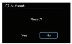
Use this module to reset all machine settings including YRC settings, display brightness, grip warmer presets, traction control, units, and all resettable vehicle information display items.
