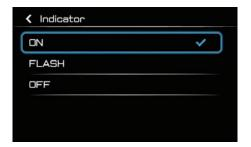
Select "ON" to have the indicator light steadily, "FLASH" to have the shift indicator flash when the indicator start threshold has been reached, or "OFF" to turn the indicator off. Confirm the settings by short pressing enter "
