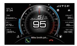
When a phone call is received to a connected smartphone, the ringtone will play through the connected headset and a telephone function will appear at the bottom of the display. Short press enter "
