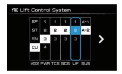
"LIF" can be set to 1, 2, and 3. Setting level 1 provides the least amount of system intervention and setting 3 most strongly reduces the amount of wheel lift. (See page 3-16.)
