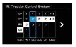
This model uses a variable traction control system. For each setting level, the farther the vehicle is leaned over, the more traction control (system intervention) is applied. There are 3 setting levels available. Level 1 applies the least system intervention, while level 3 applies the most overall traction control. (See page 3-16.)
