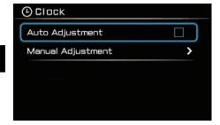
The clock can be set to auto adjust in sync with a smartphone. Auto-adjust-ment requires a connection between the CCU and the MyRide - Link app. (See page 4-1.)
