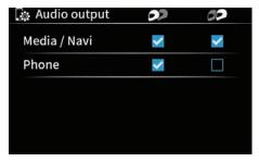
When a Bluetooth headset is connected, the headset icon "②" / "②" will appear on the top of the display. This setting module changes the media/navigation and phone call audio between the "Rider headset" "②" and "Passenger headset" "②".
