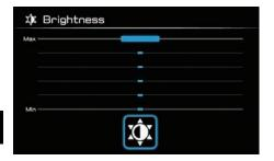
Select the brightness level of the shift indicator light from 1-6 by operating the joystick up-down. Confirm the settings by short pressing enter "✓" and return to the previous menu.
