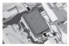
3. Remove the blown fuse using the fuse puller.
