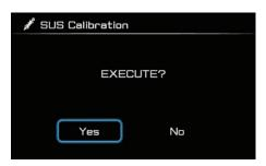
After any service to the rear suspension, a sensor calibration must be performed using this module. Select "Execute" and within approx. 10 seconds the result of the calibration (success/failed) will be displayed.
