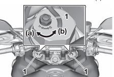
1. Spring preload adjusting nut
