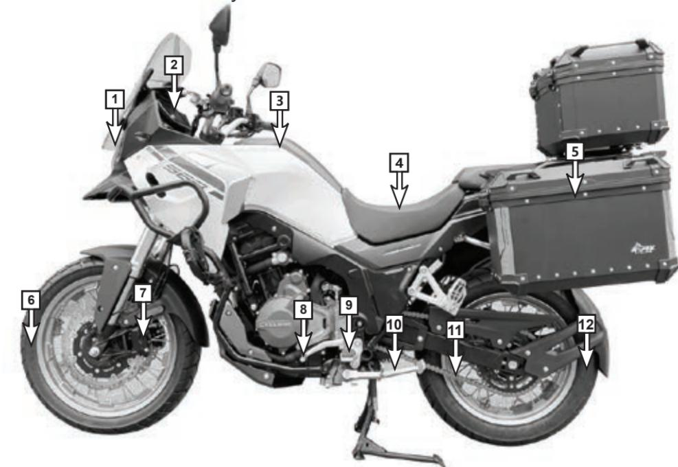
1. Headlamp 2. Instrument 3. Fuel tank 4. Seat 5. Left side box 6. Front wheel 7. Left front brake
