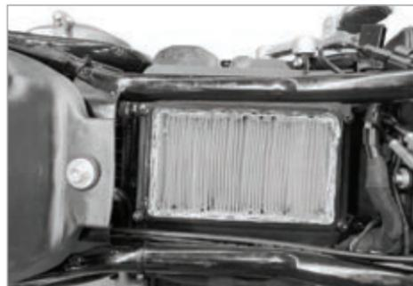
After the filter element of the air filter is blocked by dust, the resistance of the intake system will increase, the mixture is too rich, the power will decrease and the fuel consumption will increase. Therefore, the filter element should be checked, cleaned and replaced regularly.
