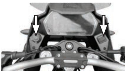
The load power of external equipment at the reserved port shall not exceed 20W; Do not refit the vehicle without authorization, otherwise, the company will not bear any consequences.
