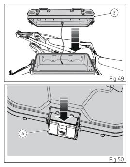
Close the cover (3) and push the lever (2) fully down, as shown in the figure. Turn the key (1) to the lock closing position. Remove the key (1).
