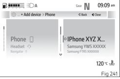
• Once confirmed, if the pairing of the device has been successful, the message "Paired" is displayed for a few seconds and then the instrument panel returns to the previous screen. Otherwise, "Pairing error" is displayed. If you are pairing an headset device, during pairing you are asked to assign the device the role of "Rider" or "Passenger":
