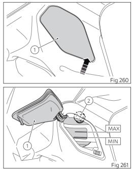
Attention This operation must be performed with cold engine. Failure to observe the above recommendation may lead to coolant or hot vapour leakage with possible consequent severe burns.
