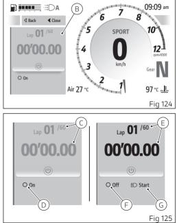
to display the time of the current lap, updating the number of laps. When the 60th lap is reached, the message "Full" is displayed and it is not possible to record new times: in this case, delete the saved laps in order to record new ones
