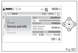
If the battery voltage is more than 16.0 volts, "HIGH" is displayed flashing in red instead of the battery data.
