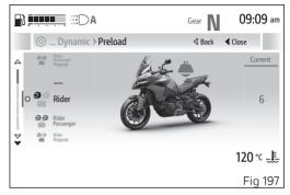
Upon accessing the sub-menu of each profile, levels 1 to 24 are displayed. The motorbike is also shown with the part involved in the setting highlighted followed by the reference indications and the currently set level.
