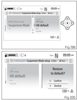
Resetting the parameter values for all Suspension Mode profiles:
