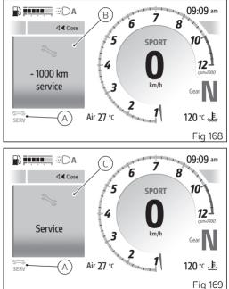
after the first 100 km (60 miles) in the case of "Oil Service" and "Valve Clearance Check Service" or for the first 10 days in the case of "Service Check", the yellow indication of the distance or days exceeded from the set threshold for the relevant service is displayed for 5 seconds.
