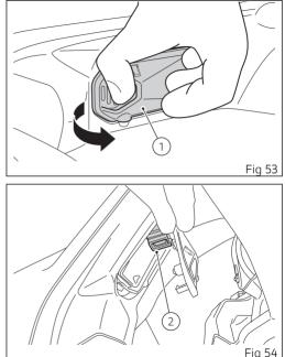
Attention The water tightness of the USB socket compartment is ensured for cables up to 3.6 mm (0.14 in) in diameter.
