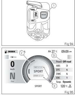
"SETUP" and press the button **O** or hold down the MODE button (1) for a long time, then you will directly access the Riding Mode Setup function in the "Settings - Advanced" menu.
