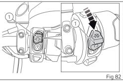
To stop the engine, move the red switch (1) downwards to the "RUN OFF" position. Turn the vehicle key off by turning the key to position (A).
