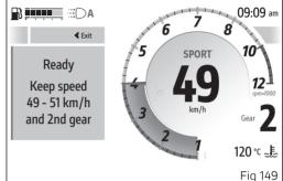
If during the calibration procedure the required speed and riding conditions are not maintained, or an error or malfunction occurs, the instrument panel displays the message "Failed" and returns to the previous menu after a few seconds.
