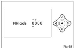
• If the PIN code is correct, the instrument panel shows "Correct" for 2 seconds, and then displays the main screen.
