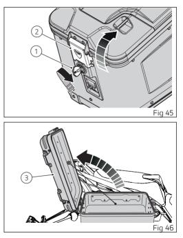
The cover (3) can be opened on both sides of the side pannier. After lifting the cover (3), press the lever (4) on the back of the side pannier, the cover (3) can be opened as shown in the figure.
