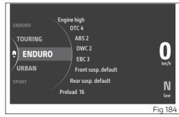
If both of the above conditions occur, the message "Close throttle and release brakes" is displayed. The new Riding Mode is confirmed and stored only when both conditions are satisfied and then the main screen is displayed.
