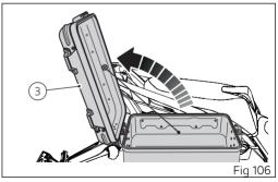
The cover (3) can be opened on both sides of the side pannier. After lifting the cover (3), press the lever (4) on the back of the side pannier, the cover (3) can be opened as shown in the figure.
