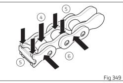
After lubrication, wait 10-15 minutes to allow the Juhricant to act on the internal and external surfaces. of the chain and then remove the excess lubricant with a clean cloth
