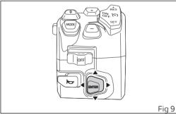
The instrument panel displays the setting screen with the currently set distance selected. Using the iovstick ▲ ▼. it is possible to scroll and select one of the 4 distances available. With the same selected distance, the higher the speed of the motorcycle, the greater the distance. The distances indicated are nominal values. Depending on the riding situation and the behaviour of the vehicle ahead, the actual distance may be less or more than these target distances:
