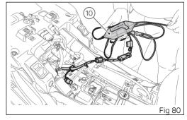
When the motorcycle is left unused (approximately for more than 30 days). We recommend owners to use the Ducati battery charge maintainer (Battery maintenance kit) since its electronics monitors the battery voltage and features a maximum charge current of 1.5 Ah. Connect the battery maintainer to the diagnostic socket.
