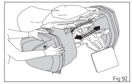
Installing the aluminium side panniers (if any)
