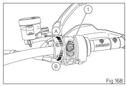
The engine will shut off by turning the red switch (1) to the "RUN OFF", position (B).
