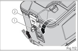
To carry out all opening / closing or installation / removal operations on the panniers, operate only the appropriate levers and never use the key to transmit force.
