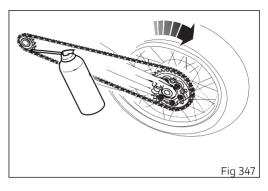
Apply the lubricant jet (1) inside the chain between the inner and outer links, in point (2) immediately before the engagement point on the sprocket.
