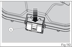
Close the cover (3) and push the lever (2) fully down, as shown in the figure. Turn the key (1) to the lock closing position. Remove the key (1).
