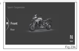
By selecting the items "Front" (Fig 235) or "Rear" (Fig 236), "Hardest", "Hard", "Medium", "Soft", "Softest" levels are displayed on the left-hand side. While the currently set level is shown on the right. The motorbike is shown in the middle with the part involved in the setting highlighted and the reference indications.
