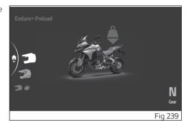
Upon accessing the sub-menu of each profile, levels 1 to 24 are displayed on the left-hand side. While the currently set level is shown on the right. The motorbike is shown in the middle with the part involved in the setting highlighted and the reference indications.
