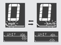
Press the MODE button. The speed and mileage unit is set, and then the display moves to the changing of the temperature gauge unit.
