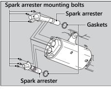
**5.** Use a brush to remove carbon deposits from the spark arrester screen. Be careful to avoid damaging the spark arrester screen. The spark arrester must be free of breaks and holes. Replace, if necessary. Check the gasket. Replace, if necessary.
