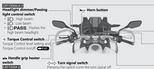
Change the handle grip heater level or turn the handle grip heater on and
