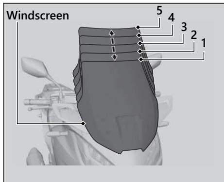
3. Check the windscreen adjustment for smooth operation and check the sliding area for looseness.
