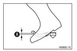
Sit on the vehicle in the riding position and determine distance between the upper edge of your boot and the shift lever.
