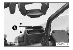
Correct the brake fluid quantity to level A.
