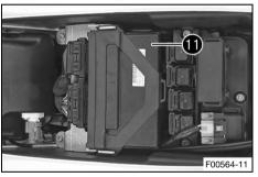
Mount engine electronics control unit 1.
