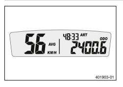
Press one of the buttons until AVG, ART and ODO appear on the combination instrument.
