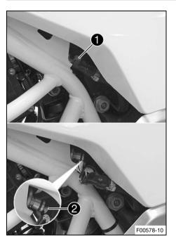
Clean quick release coupling 1 thoroughly with compressed air.
