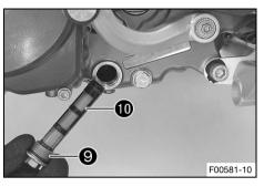
Remove screw plug 9 with oil screen 10 and the O-rings.
