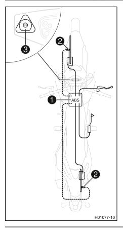
The ABS unit 1, which consists of a hydraulic unit, ABS control unit, and return pump, is installed under the seat. One wheel speed sensor 2 is located in each case on the front and the rear wheel.
