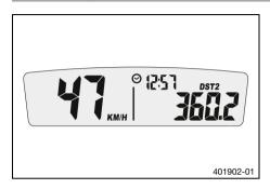
Press one of the buttons until **DST2** appears on the combination instrument.
