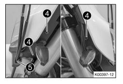
Mount and tighten screws 4.
