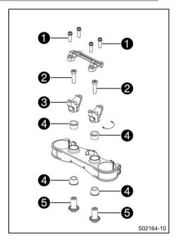
Remove screws ①. Take off the handlebar clamps. Remove the handlebar and lay it to one side.
