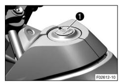
The front fuel tank is filled via fuel tank filler cap 1.
