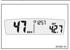
Press one of the buttons until **DST** appears on the combination instrument.
