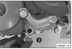
Mount and tighten screw plug with the O-ring.
