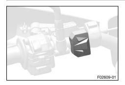
The combination switch is fitted on the left side of the handlebar.
