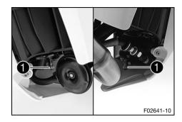
The fuel cocks **1** are located on the left/right under the fuel tank.
