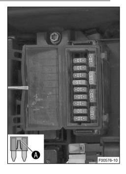
Remove the faulty fuse.
