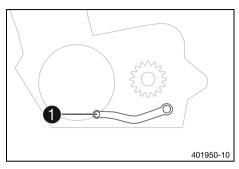
The shift lever **1** is mounted on the left side of the engine.
