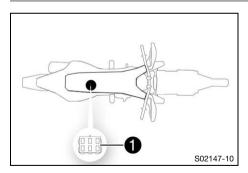
Diagnostics connector 1 is located under the engine electronics control unit.
