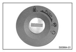
The ignition and steering lock is located in front of the seat.
