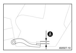
Move the foot brake lever back and forth between the end stop and the contact to the foot brake cylinder piston and check free travel **A**.
