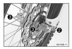
Clean and grease the wheel spindle.
