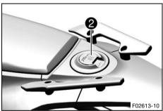
The rear fuel tank is filled via fuel tank filler cap 2.
