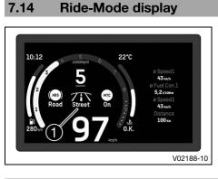
The **<u>Ride Mode</u>** setting is shown in area **()** of the display. The riding mode can be configured in the menu **Ride Mode**.
