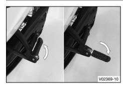
The passenger foot pegs can be folded up and down.
