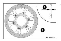
Check front and rear brake disc thickness at multiple points for the dimension  $(\mathbf{A})$ .
