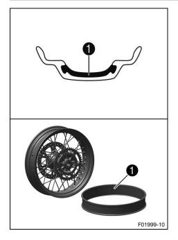
This vehicle uses a tubeless tire system in which a rim seal band **①** is used instead of the conventional tube.
