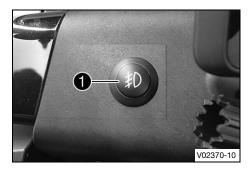
Supplementary headlight switch **1** is located on the left, next to the combination instrument.
