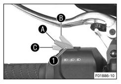
The light switch **1** is fitted on the combination switch on the left.
