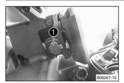
USB socket ① for the power supply to external devices is mounted on the left side of the mask support. The USB socket is activated when the ignition is switched on.
