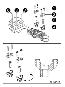
Remove screws **1**. Take off the handlebar clamps **2**. Position the handlebar so that screws **3** are accessible.
