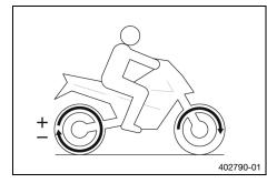
The spin adjuster is a motorcycle traction control function. The slip adjustment allows the motorcycle traction control to be tuned through nine levels to the desired characteristic map. Level 1 allows the maximum slip on the rear wheel, and level 9 the minimum.
