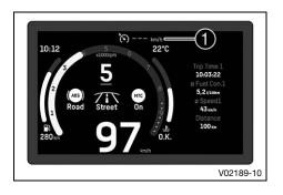
The operating state and active cruise control are shown in the **1** area of the display.
