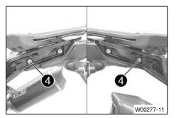
Mount and tighten screws 4.
