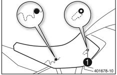
Attach the front rider's seat to the fuel tank at the recesses ①, and push the front rider's seat down and forward at the same time.
