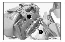
To remove the bag, press locking clips ① away from the rack.
