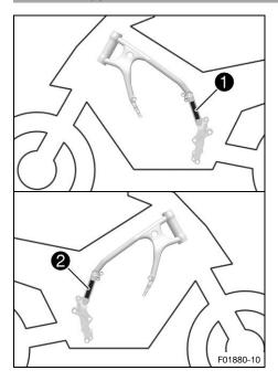
The type label **1** is located on the frame on the left. The type label for Australia **2** is located on the frame on the right.
