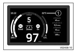
The ambient temperature is shown in area 1 of the display. The ambient air temperature is displayed in °C or °F. The unit of the ambient air temperature can be configured in the Units menu.
