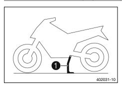
In addition to the side stand, the vehicle is equipped with a center stand **①**.
