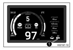
The status of the grip heater is shown in area **1** of the display. The grip heater can be configured in the **Heating** menu.
