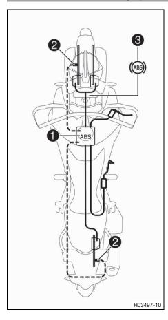
The <u>ABS</u> module **1**, which consists of a hydraulic unit, ABS control unit, and return pump, is installed under the fuel tank. One wheel speed sensor **2** is located in each case on the front and the rear wheel.
