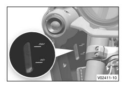
Add coolant until the coolant reaches the specified level. Guideline
