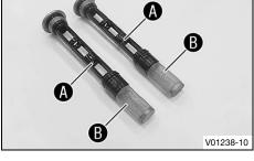
Mount the oil drain plugs 2 with magnets and new seal rings, and tighten.
