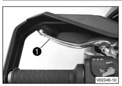
Clutch lever 1 is fitted on the handlebar on the left.
