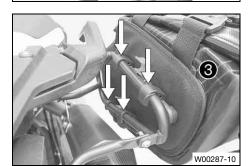
Position right side bag brackets ③ above and below on the side bag rack and press downwards until they are firmly seated on the rack.
