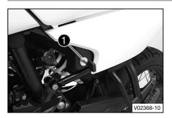
Seat lock **1** is located on the left side of the vehicle. It can be unlocked using the ignition key.
