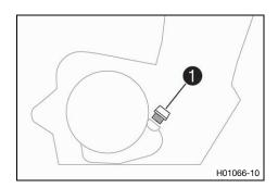
Mount and tighten filler plug 1 with the O-ring.
