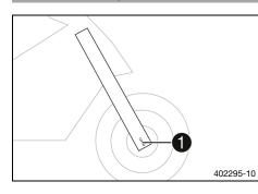
The fork part number **1** is stamped on the inner side of the fork stub.
