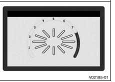
The shift light is integrated in the rpm gauge display. In the **Shift Light** submenu, the engine speed for the shift warning light can be set. The shift warning light is always active during the running-in phase (up to 1,000 km / 621 mi). The shift warning light can only be deactivated, and the values for **RPM1** and **RPM2** can only be adjusted after this. At **RPM1**, the engine speed display flashes, and at **RPM2** the entire display flashes
