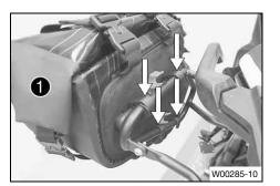
Position left side bag brackets ① above and below on the side bag rack and press downwards until they are firmly seated on the rack.
