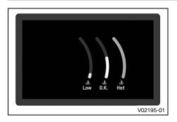
The coolant temperature indicator is a bar. The higher the bar is filled, the hotter the coolant.
