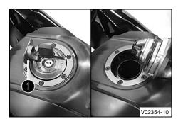
Lift cover **①** of the fuel tank filler cap and insert the ignition key into the lock.
