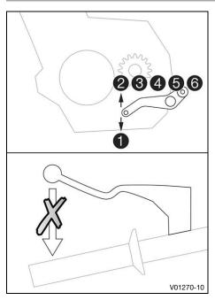
If Easy Shift is activated, you can shift up and down without operating the clutch.
