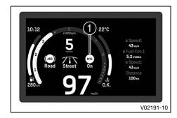
The **1** area of the display indicates whether **MTC** (IP p. 149) is switched on or off.
