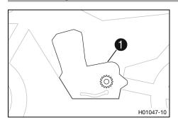
The engine number 1 is stamped onto the engine case at the top.
