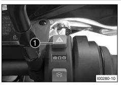
The hazard warning flasher switch **1** is fitted on the right side of the switch.
