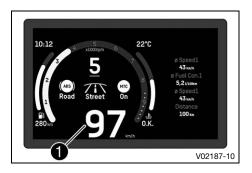
The speed is shown in area 1 of the display. Speed is shown in kilometers per hour km/h or in miles per hour mph. The unit of speed can be configured in the **Units** menu.
