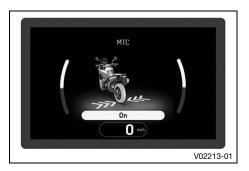
The motorcycle traction control (MTC) lowers the engine torque in case of loss of traction in the rear wheel. Depending on the riding mode, different amounts of slip are allowed when traction control is activated.
