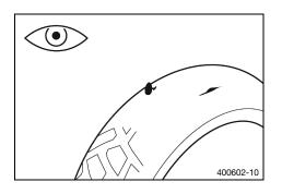
Check the front and rear tires for cuts, embedded objects, and other damage.
