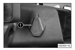
Socket **1** for electrical accessories is located on the right, next to the combination instrument.
