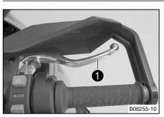
The hand brake lever ① is fitted on the right side of the handlebar. The front brake is engaged using the hand brake lever.
