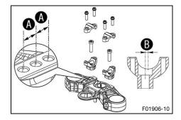
On the upper triple clamp, there are three holes at a distance of  $igadeble{A}$  to each other.
