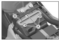
A. Air Cleaner Element Cap Screws B. Air Cleaner Element Cap
