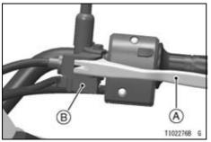
A. Clutch Lever B. Starter Lockout Switch
