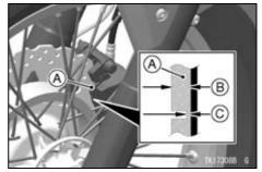
A. Front Brake Pads B. Lining Thickness C. 1.5 mm (0.06 in.)
