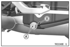
A. Engine Oil Drain Bolt B. Gasket
