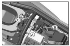
A. Fuse Boxes B. Fuse Box (ABS) C. Main Fuse
