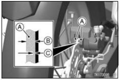
A. Rear Brake Pads B. Lining Thickness C. 1.5 mm (0.06 in.)
