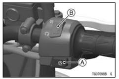
A. Starter Button B. Engine Stop Switch
