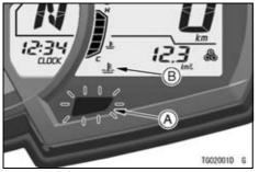
A. Warning Indicator (Red) B. Coolant Temperature Warning Indicator
