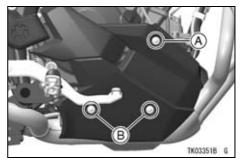
A. Lower Fairing Bolt (Upper) and Collar B. Lower Fairing Bolts (Lower) and Collars
