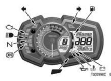
When the ignition switch is turned on, all indicators go on/off as shown in the table. If any indicator does not operate as shown, have it checked by an authorized Kawasaki dealer.
