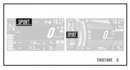
The current setting of the integrated riding mode is shown. Refer to the Integrated Riding Modes section in the HOW TO RIDE THE MOTORCYCLE chapter (see page 188).
