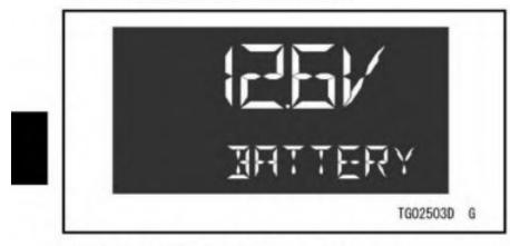
To display the battery voltage:
