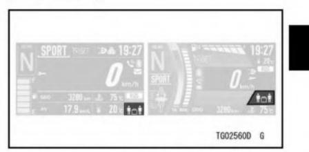
The current setting of the KECS spring preload is shown. Refer to the KECS section in the HOW TO RIDE THE MOTORCYCLE chapter (see page 202).
