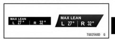
This shows the maximum lean angles of the vehicle by numerical value. *How to Reset*
