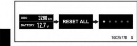
Flow when pushing and holding RE-SET button
