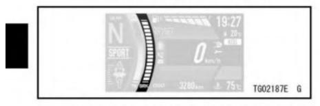
The fluid pressure of the front brake line is shown.
