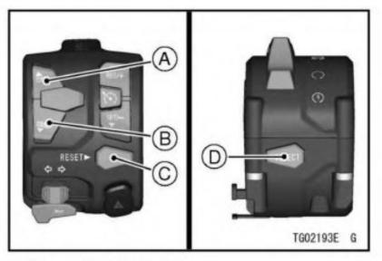
A. Upper MODE Button B. Lower MODE Button C. RESET Button D. SELECT Button
