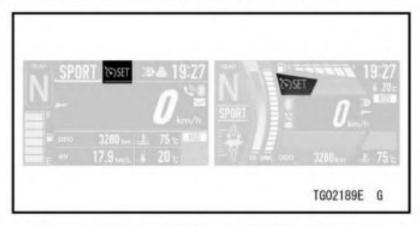
The status of the electronic cruise control system is shown. Refer to the Electronic Cruise Control System section in the HOW TO RIDE THE MO-TORCYCLE chapter (see page 208).
