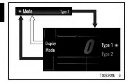
: Flow when pushing SELECT button : Flow when pushing RESET button
