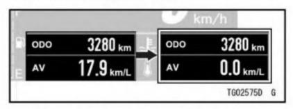
Flow when pushing and holding RE-SET button
