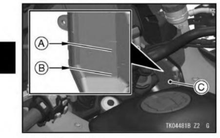
A. F (Full) Level Line B. L (Low) Level Line C. Reserve Tank  If the amount of coolant is insufficient, add coolant into the reserve tank.
