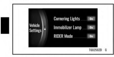
Cornering Lights: Turn cornering light system on or off
