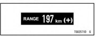
This indicates the cruising range from the remaining fuel in the fuel tank.
