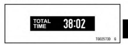
This shows the amount of time that has elaped while the ignition switch is turned on.
