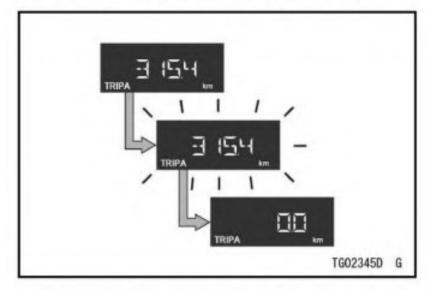
Flow when pushing and holding reset button
