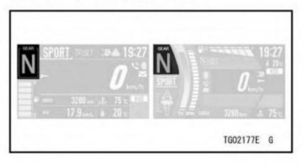
The current gear position is shown. When the transmission is in neutral, "N" appears.
