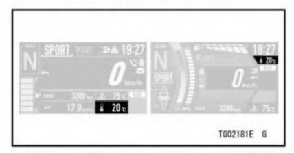
The outside temperature around the vehicle is shown.
