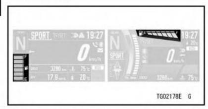
The fuel level in the fuel tank is shown by the number of segments displayed between E (empty) and F (full).
