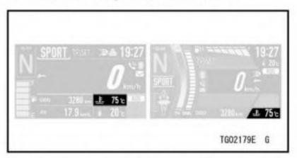
This meter shows the coolant temperature. The meter display is as shown below.
