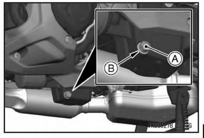
A. Engine Oil Drain Bolt B. Gasket
