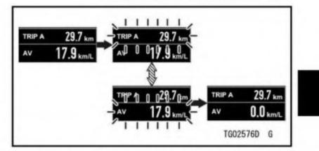
: Flow when pushing and holding RE-SET button
