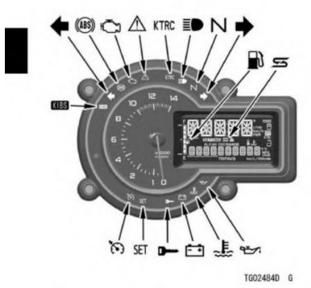
When the ignition switch is turned on, all indicators go on/off as shown in the table. If any indicator does not operate as shown, have it checked by an authorized Kawasaki dealer.
