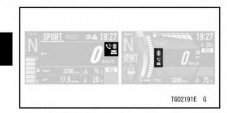
The Bluetooth icon appears when your smart device is connected to the vehicle. The telephone icon appears when a phone call is received by your smart device. The mail icon appears when a email or text message is received.
