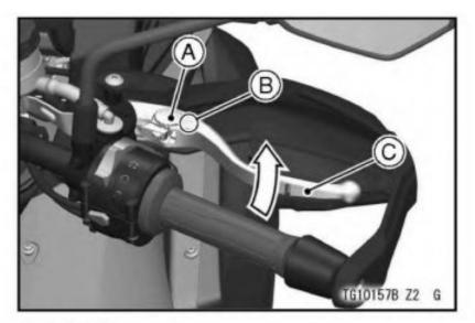
A. Adjuster B. Mark C. Brake Lever
