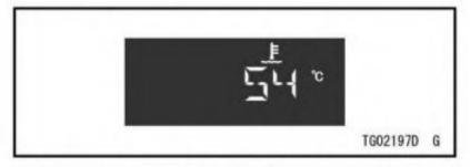
This meter shows the coolant temperature. The meter display is as shown below.
