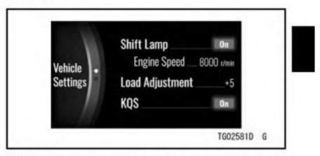
Shift Lamp: Turn shift-up indicator system on or off
