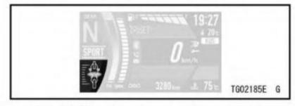
This indicator shows the acceleration/deceleration rate of the vehicle. When acceleration is greater, the indicator moves more to the back side of the vehicle illustration. When deceleration is greater, the indicator moves more to the front side of the vehicle illustration.
