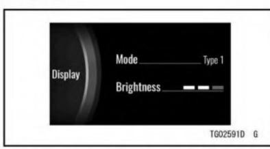
Mode: Switch layout of LCD Brightness: Adjust backlight of LCD
