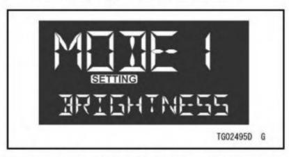
Push the select button. The current setting starts blinking.
