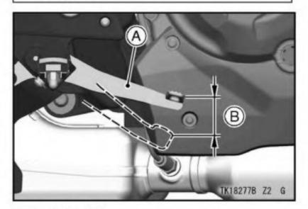
A. Brake Pedal B. Brake Pedal Travel
