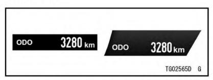
The odometer shows the total distance. This meter cannot be reset.
