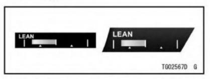
This shows the lean angle of the vehicle. The more it is leaned, the larger the bar on the gauge. **Maximum Lean Angles**
