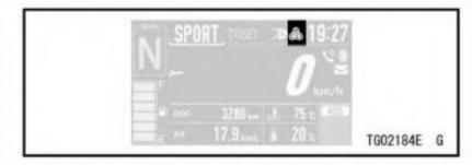
When riding the motorcycle efficiently, the economical riding indicator appears on the LCD to indicate favorable fuel consumption. Monitoring the economical riding indicator can help the rider maximize fuel efficiency.
