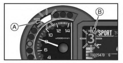
A. Shift-up Indicator (Blink) B. Gear Position Indicator (Change in Color)
