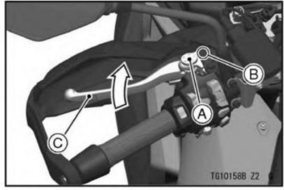
A. Adjuster B. Mark C. Clutch Lever
