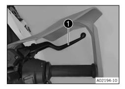
The front brake is engaged using the hand brake lever.
