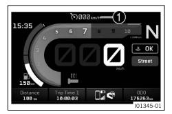
The operating state of the activated speed control (optional) is shown in display area **1**.
