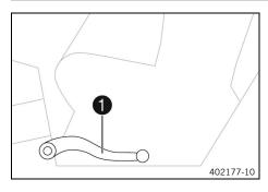
The rear brake is operated with the brake pedal.
