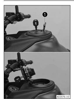
Lift cover 1 of the fuel tank filler cap and insert the ignition key into the lock.
