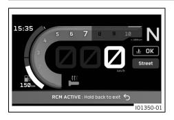
The **Remote Control Mode** indicator (optional) appears when **Remote Control Mode** is activated.
