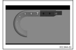
The shift warning light is integrated in the display.
