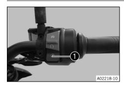
Electric starter 1 is fitted on the right side of the handlebar.
