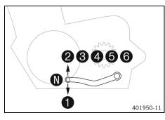
The gear positions can be seen in the figure.
