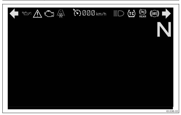
The indicator lamps offer additional information about the operating state of the motorcycle. When the ignition is switched on, all indicator lamps light up briefly, except for the TC indicator lamp (a).
