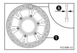
Check the brake disc thickness of the front and rear brake disc at several places on the disc to see if they conform to measurement A.
