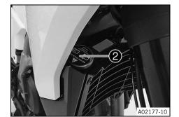
Remove radiator cap 2 and check the coolant level in the radiator.
