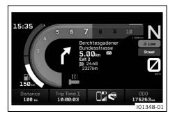
The **Navigation** indicator (optional) appears when the navigation function is activated.
