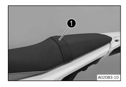
Passenger strap 1 is mounted on the seat.
