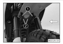
Position the front fender. Mount and tighten screws 1.
