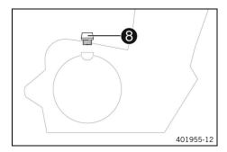
Remove filler plug (3) with the O-ring, and fill up with engine oil.
