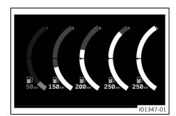
The fuel level display consists of the fuel range display and a bar. The higher the bar is filled, the more fuel there is in the fuel tank.
