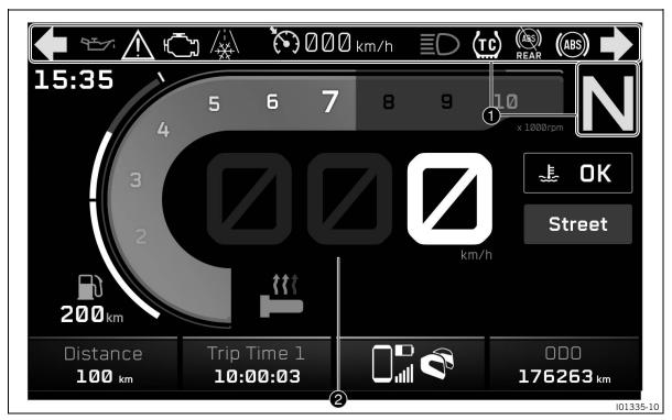
The combination instrument is attached in front of the handlebar.  $\label{eq:combination}$
