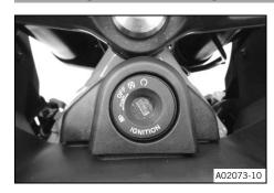
The ignition and steering lock is located in front of the upper triple clamp.
