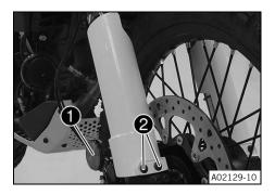
Position the fork protector. Mount screw ①, but do not tighten yet.
