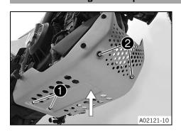
Position the skid plate, mount and tighten screws 1 and 2. Screw, engine guard M6 9 Nm (6.6 ft·lb<sub>f</sub>) Loctite® 243
