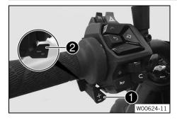
The **+RES** button **1** is fitted on the front left of the handlebar.
