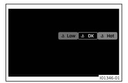
The coolant temperature is displayed by a symbol. The symbol changes between **LOW**, **OK** and **HOT** depending on the temperature.
