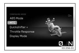
In the combination instrument, the motorcycle traction control can be switched on or off via the **MTC** submenu (optional).
