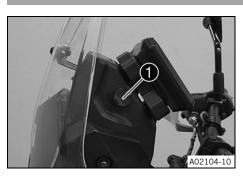
A USB socket 1 is located in the storage compartment for supplying power to external devices.
