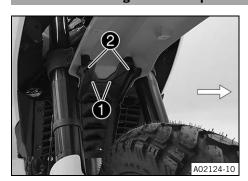
Remove screws 1 and 2. Take the fender off to the front.
