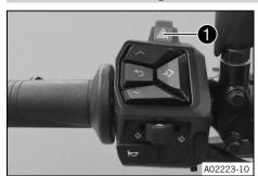
The hazard warning flasher switch **1** is fitted on the top of the combination switch.
