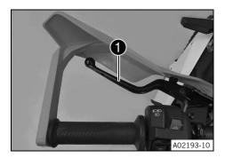
Clutch lever 1 is fitted on the left side of the handlebar.
