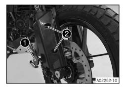
Position the fork protector. Mount screw with the reflector, but do not tighten yet.
