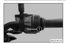
Electric starter 1 is fitted on the right side of the handlebar.
