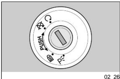
The light switch turns off when the ignition switch is set to «KEY OFF».
