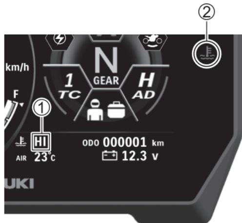
If the engine coolant temperature warning indicator light comes on, stop the motorcycle in a safe place, perform the following checks, and take any necessary action.
