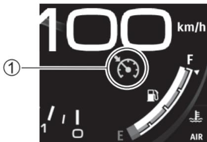
2. With the cruise control indicator ① on, press CRUISE SPEED switch **SET/-** ② in the left handlebar switch area after reaching the set speed to set the cruise control speed to maintain the current speed after relaxing the throttle grip. The cruise control SET indicator ③ turns on after setting a speed.
