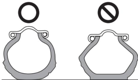
Check tire pressure each day before you ride, and be sure the pressure is correct for the vehicle load according to the chart below.
