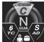
3. The Suzuki drive mode selector indicator indicates the selected mode.
