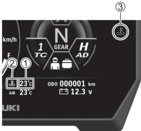
The following information appears when the engine coolant temperature is not 20°C (68°F) or more and less than 120°C (248°F).
