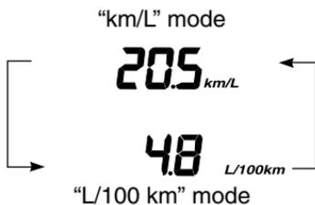
Set the meter ⑰ to instantaneous fuel consumption meter or average fuel consumption, then press and hold the MODE switch (Down) for 2 seconds to change "km/L" mode to "L/100 km" mode.
