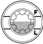
4. Hold the motorcycle vertically and check the oil level through the oil level inspection window on the right side of the engine. The engine oil level should be between "L" (low) and "F" (full) lines.
