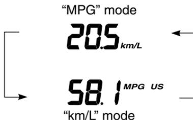
Set the meter ⑳ to odometer, then press and hold the ADJ button ① for 2 seconds to change "MPG" mode to "km/L (L/100 km)" mode. At the same time, the odometer will be change between mile and km.
