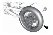
NOTE: Never depress the rear brake pedal with the rear wheel removed. It is very difficult to force the pads back into the caliper assembly.
