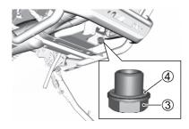
12. Pour 3.7 US qt (3500 ml) of new engine oil through the filler hole and install the filler cap. Be sure to always use the specified engine oil described in the "SELECTING THE ENGINE OIL" section on page 3-29.
