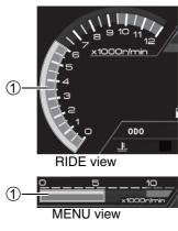
Ex: RPM setting 6,000 r/min
