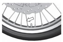
To tighten the spoke nipples properly, tighten them equally to the specified torque. Loosened and overtightened spoke nipples may cause unequal tension of spokes and may result in distortion of the wheel rim. Contact your dealer to perform this service.
