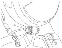
1. Headlight assembly mounting bolt
