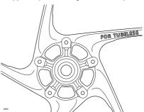
Typical Wheel Marking - Tubeless Tyre
