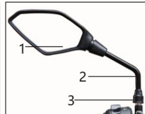
The fastening torque for nut 3:40Nm
