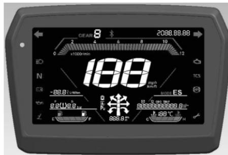
Under the mode of ODO, long press the lower key can shift the unit between Imperial/Metric for Speed/Mileage; When got into mode TRIP, long press lower key to erase the record for single mileage. In normal displaying page, short press upper key to shift Voltage/Temperature/Fuel consumption in turn. (Default is showing temperature).
