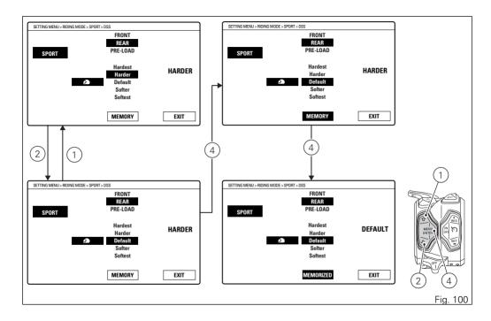
Adjustment of the rear shock absorber spring preload
