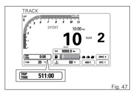
If you change the unit of measurement for an item connected to Speed (and distance) or Consumption or after a Battery-OFF, the trip time value will be automatically reset.
