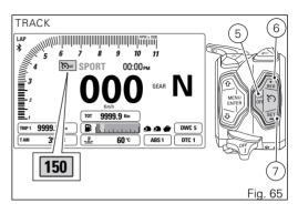
Once the system is enabled, it is possible to set the current speed as the desired speed by pressing RES (6) or SET (7): press RES (6) if no target speed has been previously set.
