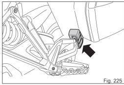
Push forward (towards the front wheel) until fully home; only in this position will it be possible to lower handle and lock pannier in place, this operation ensures pannier locking to its mounting points. Turn the key counter clockwise to lock handle and remove it.
