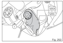
This type of mixture ensures the best operating conditions (the coolant starts to freeze at -20 °C/-4 °F). Cooling circuit capacity: 2.5 cu. dm (litres).
