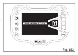
Warning reading "Steering locked" (upon Key-Off)
