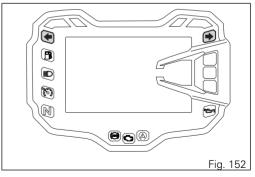
Once the "Hazard" function is activated, if vehicle is turned off (key turned to "OFF"), the function stays active for 2 hours. After 2 hours, the turn indicators switch OFF automatically in order to save battery charge.
