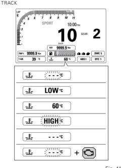
If the coolant temperature sensor is in fault, a string of flashing dashes "---" is displayed with the set unit of measurement and the MIL light turns on. If the instrument panel is not receiving coolant temperature value, a string of steady dashes "---" is displayed, followed by the unit of measurement.
