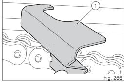
To measure the proper chain tensioning, it is necessary to check the correspondence of the chain pin axis (black line in (Fig. 267)), within the distance identified with the cutout on chain tension gauge (interval indicated by the arrows in (Fig. 267)). If chain pins are higher or lower than this interval (Fig. 268), it is necessary to tension the chain page 359.
