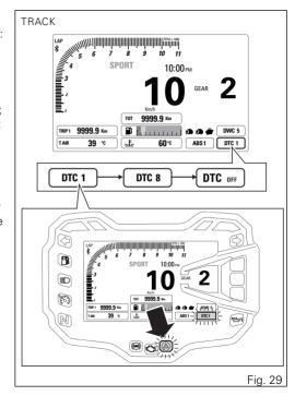
If DTC is in fault or the Black Box is in fault, the instrument panel will display DTC Err and DTC/DWC warning light will be steady on.
