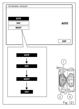
Select DAY (day mode) to permanently set display "white" background for improved readability - recommended in conditions of strong ambient light. Select NIGHT (night mode) to permanently set display black background for dimmed visibility - recommended in case of poor ambient light and/or at night.
