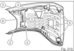
Fit the passenger seat on the motorcycle. Now the seat is in a lowered position.
