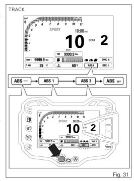
If the ABS is in fault, the instrument panel will display ABS Err and ABS warning light will be steady on.
