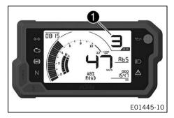
The current gear is shown in area 1 of the display.
