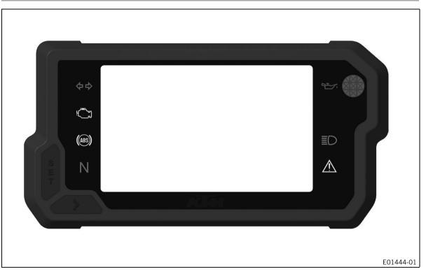
The indicator lamps offer additional information about the operating state of the motorcycle. When the ignition is switched on, all indicator lamps light up briefly except for the turn signal indicator lamp. As soon as a warning for operating safety has been detected, the general warning lamp (a) also lights up.
