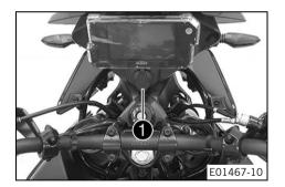
Socket **①** for electrical accessories is fitted in front of the upper triple clamp.
