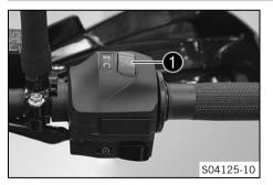
The emergency OFF switch  $\bigcirc$  is fitted on the right side of the handlebar.
