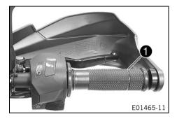
The throttle grip ① is fitted on the right side of the handlebar.
