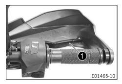
The hand brake lever  $\bigcirc$  is fitted on the right side of the handlebar.
