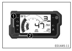
Press the **SET** button ① to change display modes. Possible display modes are **ABS Modus**, **Info**, distance 1 (**TRIP 1**) and distance 2 (**TRIP 2**).
